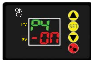
P4=ON=AUTO Timing Cycle Starts at Power On PV \approx 0, SV \approx 0
